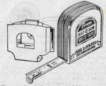
Chrome plated die cast case. ½ inch tempered steel blade finished with bonderized white enamel both sides. Easy-to-read jet black "quick-conversion" foot and inch markings on blade which is marked in eighths and sixteenths, thirty-seconds on first six inches. Self-adjusting end hook slides to compensate for its thickness, assuring accurate inside and outside measurements. Blade easily replaced without tools. Holster, complete with belt clip, included with each tape.
