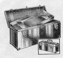
Lift out tray can be removed from box for convenience and adaptability to other uses. Heavy gauge steel throughout, double lock seamed construction. Reinforced corners at bottom. Rounded cover with embossed stripes. Heavily plated drawbolts with built-in padlock eye. Full length, piano type hinge. Indestructible rust proof formed steel handle. Hard baked blue enamel inside Exterior silver detone. Two coat finish outside:
