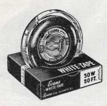
Heavily zinc plated steel case covered with a heavy leather grained DuPont vinyl, fully resistant to moisture, scuffs and stains, held by stainless steel edge band. Strong die-cast zinc winding reel with housing, recessed crank and double roller mouthpiece, heavily chrome plated. Improved anti-backlash winding. Snow white bonderized steel 3/8 inch tape with jet black markings and hook ring.
